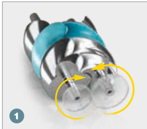
1 Intake air is captured
